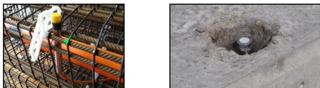
Figure 3. Piezometer in test pile (left/right: before/after casting).
